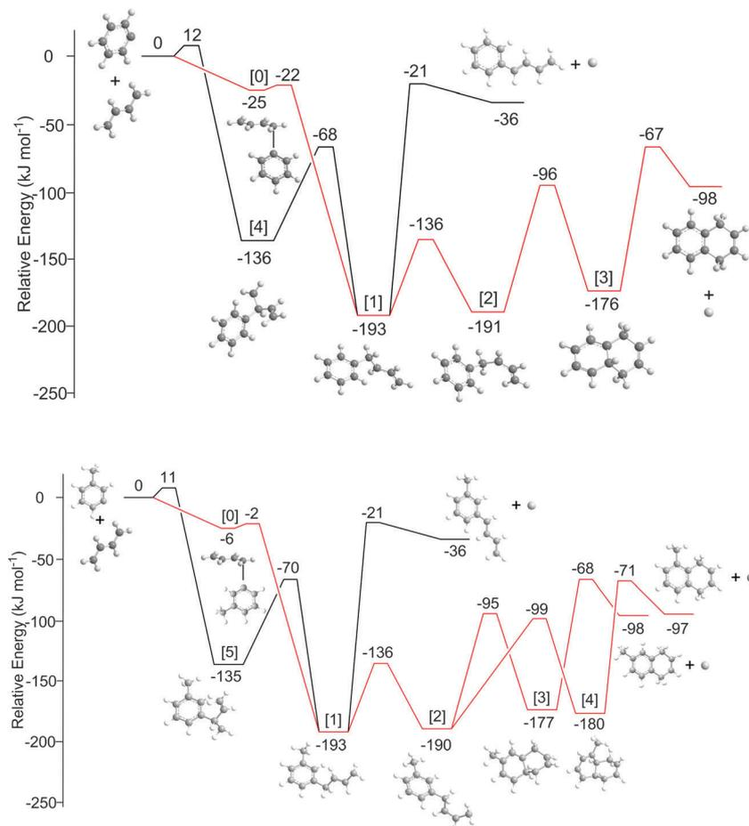
Fig. 5 Potential energy surface for the reaction of the *meta*-tolyl radical with 1,3-butadiene (bottom) in comparison to the potential energy surface of the phenyl-1,3-butadiene reaction (top). Energies for intermediates, transition states, and products are given relative to the reactants energy (in  $\text{kJ mol}^{-1}$ ) at the G3(MP2,CC)//B3LYP/6-311G\*\* level of theory.
