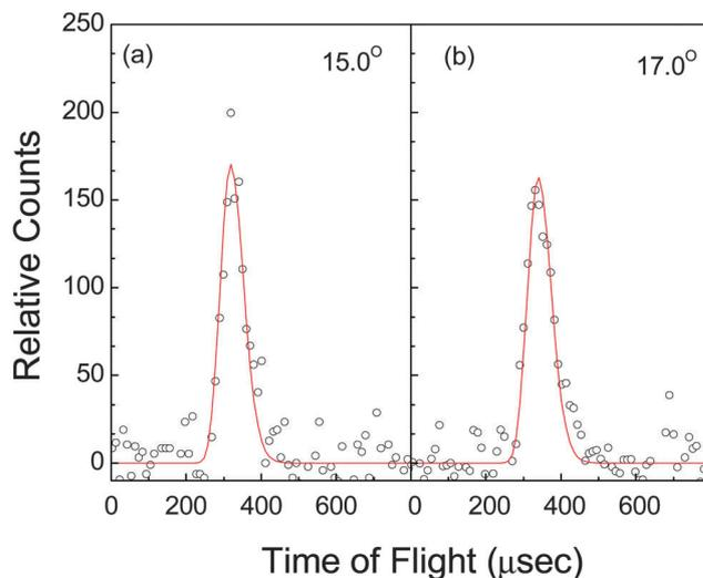
Fig. 3 Time-of-flight data recorded at the center-of-mass for the atomic hydrogen loss pathway in the reaction of *meta*-tolyl ( $C_7H_7$ ) with 1,3-butadiene ( $C_4H_6$ ) recorded at  $m/z$  144 ( $C_{11}H_{12}^+$ ) (a) and D6-1,3-butadiene ( $C_4D_6$ ) recorded at  $m/z$  150 ( $C_{11}H_6D_6^+$ ) (b), respectively. The circles present the experimental data and the red lines present the fits utilizing the best fit center-of-mass functions.
