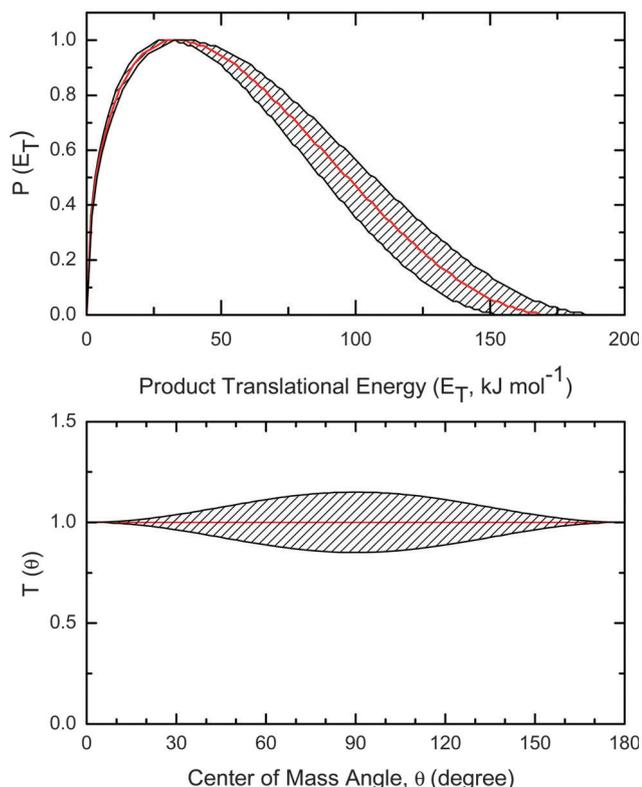
Fig. 4 Center-of-mass translational energy distribution (top) and angular distribution (bottom) for the reaction of *meta*-tolyl ( $C_7H_7$ ) with 1,3-butadiene ( $C_4H_6$ ) to form ( $C_{11}H_{12}$ ) plus atomic hydrogen. The hatched area represents the possible fits that remain within the error boundaries of the LAB angular distribution shown in Fig. 2.
