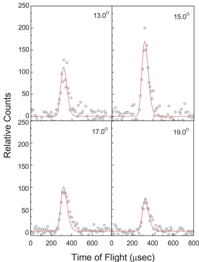
Fig. 1 Time-of-flight data at various laboratory angles for the reaction of the *meta*-tolyl (C<sub>7</sub>H<sub>7</sub>) with 1,3-butadiene (C<sub>4</sub>H<sub>6</sub>) recorded at *m/z* 144 (C<sub>11</sub>H<sub>12</sub><sup>+</sup>) at a collision energy of 48.5 ± 3.5 kJ mol<sup>-1</sup>. The circles represent the experimental data and the red lines the fits.
