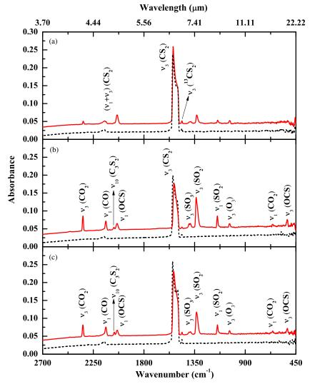
**Figure 1.** Infrared spectra of carbon disulfide (CS<sub>2</sub>)–oxygen (O<sub>2</sub>) ices at 12 K before irradiation (dashed trace) and after irradiation (solid trace) at three different currents of the electron beam: (A) 100 nA (3 hr) (B) 1000 nA (1 hr) and (C) 5000 nA (1 hr). (A color version of this figure is available in the online journal.)
