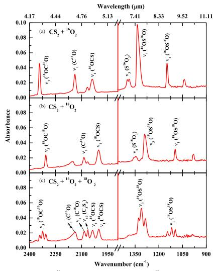
**Figure 2.** Infrared spectra of (A) carbon disulfide (CS<sub>2</sub>) +  ${}^{16}O_2$  (1:15) ices, (B) carbon disulfide (CS<sub>2</sub>) +  ${}^{18}O_2$  ices, and (C) carbon disulfide (CS<sub>2</sub>) +  ${}^{16}O_2$  +  ${}^{18}O_2$  ices after irradiation at 1000 nA of the electron beam (1 hr) at 12 K. (A color version of this figure is available in the online journal.)
